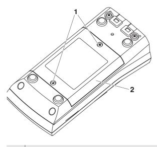
3 Place four batteries (type Mignon AA) in the battery compartment.
