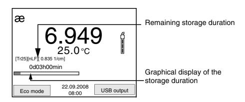
The active automatic storage function can be recognized from the progress bar in the status line. The progress bar indicates the remaining storage duration.
