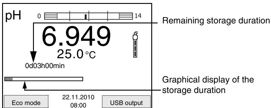
The active automatic storage function can be recognized from the progress bar in the status line. The progress bar shows the remaining storage duration.
